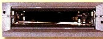
**PCMCIA (Personal Computer Memory Card International Association)** slots are found on portable computers. Devices that fit in these slots are called PC Cards. There are three types of PC Cards: Type I, Type II, and Type III. CardBus is a variation on the PCMCIA standard that supports a 32-bit bus (wider than the PCMCIA original of 16 bits), and bus mastering and operation speeds up to 33 MHz.
