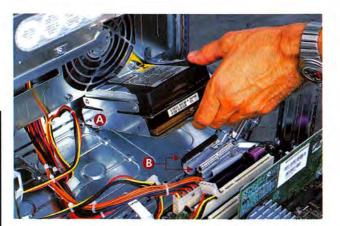
Slide the whole drive carrier into the computer case, lowering the back of the carrier in first
