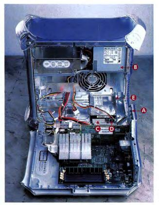
After you've unplugged your Power Mac, open its case using the latch on the side panel. Ground yourself by touching the metal on the PCI port covers (a) or the power supply box (B). (Once you've done this, don't go walking around the room in your socks; stay put until you're done.)
