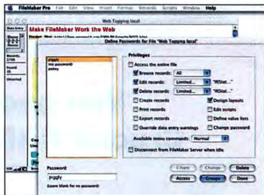
Access Privileges FileMaker Pro 5.5's Passwords dialog box lets you restrict access on a record-by-record basis.
