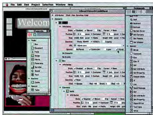
Inside and Out iShell's nested outlines, which replace the timelines of other authoring tools, help reduce complexity.
