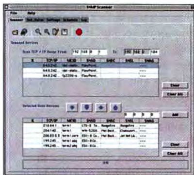
Scan Your WAN Asset Trustee's SNMP Scanner monitors ranges of IP addresses.
