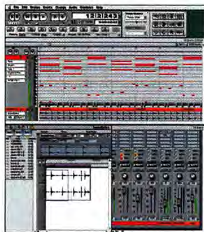
Digital Performing Digital Performer 3.0.1's Sequence Editor (middle window) lets you edit audio and MIDI data in one place. Also shown are the Control Panel window (top) and the new Soundbites and Mixing Board windows (bottom).
