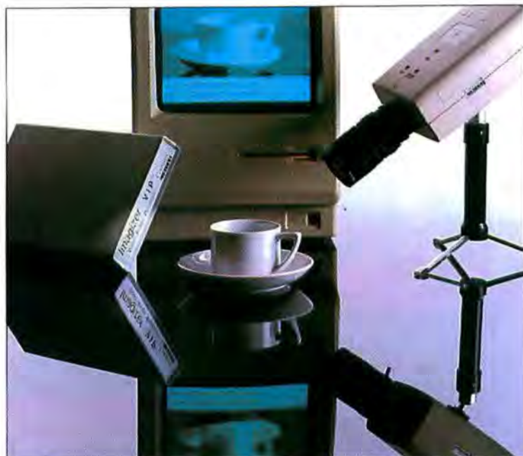
The Imagizer from Comtrex Limited allows you to store video input as PostScript files on the Mac and to print images with a 256-level gray scale.
