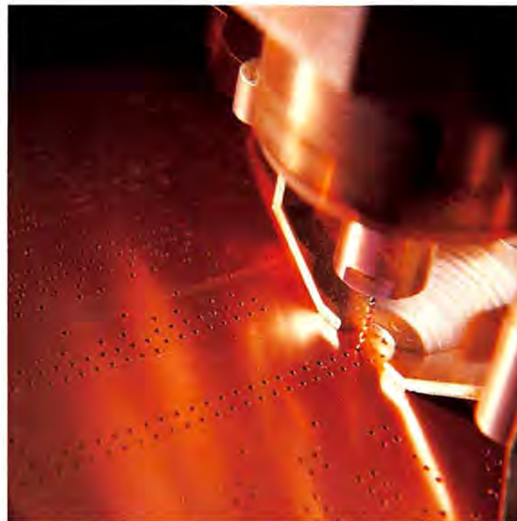
Following instructions from a nearby Macintosh, this machine drills holes in a printed circuit board also designed on a Mac.
