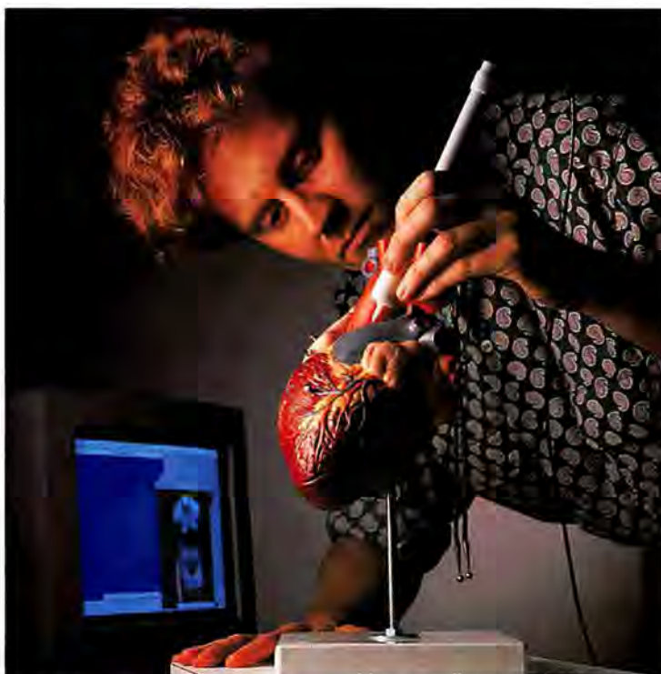
Dan Donaldson uses Mira Imaging's 3-D probe, which images and rotates three-dimensional shapes, to define the surface of a heart model to a nearby Macintosh.
