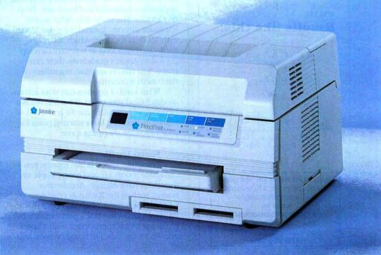
The DirectPrint non-impact page printer works with both Apple and MS/DOS-based systems. Weighing only 35.2 pounds, it is 15.7" wide by 13.4" deep by 9.1" high.
