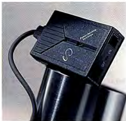
Silver Streak 10-Mbps Ethernet transceivers make installation relatively simple by using standard silver-satin phone wire.
