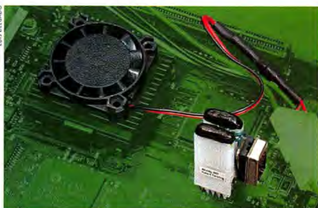
Boosted Centris 610 To make a Centris 610 run faster involves clipping a faster oscillator (highlighted at right) onto the 610's clock crystal and then adding a heat sink and cooling fan to the 610's CPU (highlighted at left).
