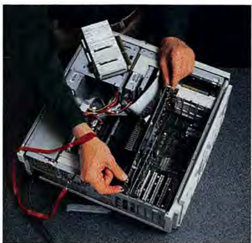
Too Tight a Squeeze One problem we discovered: you can't install a VideoVision PCI card from Radius in a Umax clone because the daughtercard takes up too much space. Radius and Umax have collaborated on a workaround to solve this.
