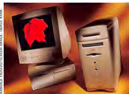
The Power Mac 4400 (left) features a desktop enclosure, while the Power Mac 6500 is a tower system.
