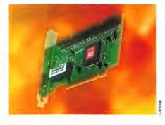
drives. In a four-drive configuration, two drives must be set up as *masters* and the other two as *slaves*. As you add slave devices, the system slows down. In our tests, a configuration with two master drives was generally 10 percent faster than a master-and-slave configuration.
