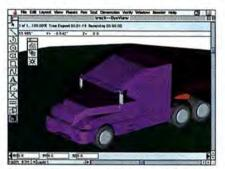
Honk! Here's AutoCAD's famous truck file, translated into Vellum Solids '99 from .DXG and rendered with Vellum's own lighting and shadowing effects.
