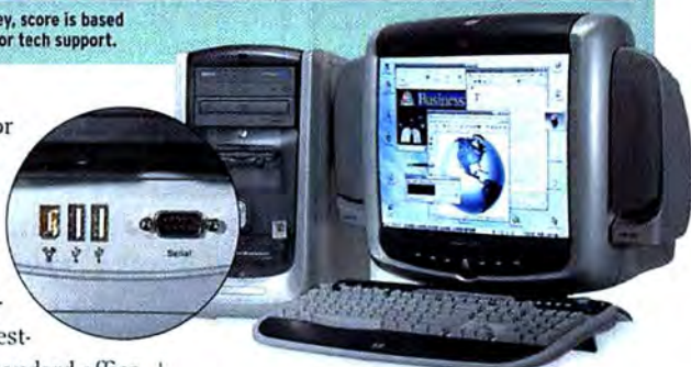
UP-FRONT ACCESS: HP's Pavilion 7875 has IEEE-1394, USB, and serial ports.
