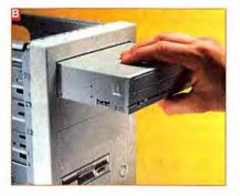
the case, you may have to attach mounting brackets that came with the case. Some cases don't require them. When you install the drives, make sure that their fronts line up with the front of the case (B).
