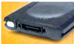
Read/write heads are integrated into each fully sealed Peerless disk, drastically reducing the risk of contamination.
