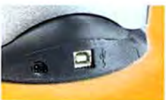
The Peerless drive supports modular connectivity—you can switch between FireWire® and USB interfaces.
