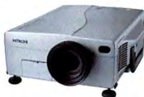
HITACHI'S CP-SX5500W is the company's first projector to utilize LCOS technology.
