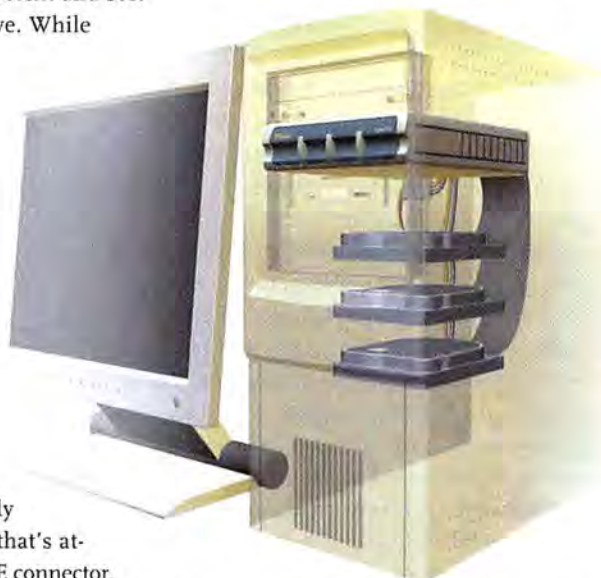
FIGURE 1: THE TRIOS RX-910T6 hard drive selector isolates your files on a shared PC.
