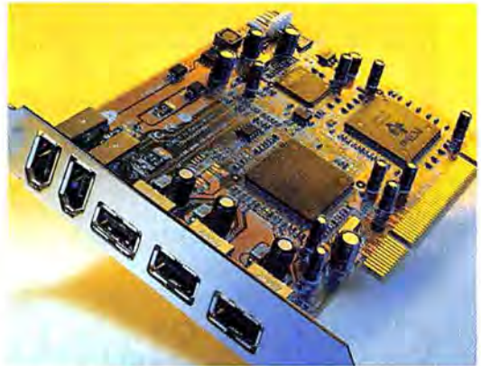
FIGURE 2: TWO IN ONE! A USB 2.0/IEEE 1394 combo card takes up just one PCI slot.
