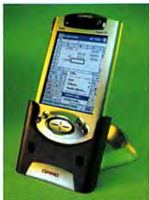
HP'S IPAQ 3950 features Intel's new CPU, the PXA250.
