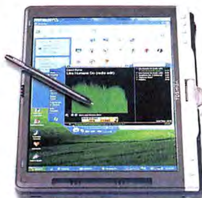
NOTEBOOKS like Toshiba's Portégé 3500 look like normal laptops, but with a twist and flip of the screen, they're tablet-ready.
