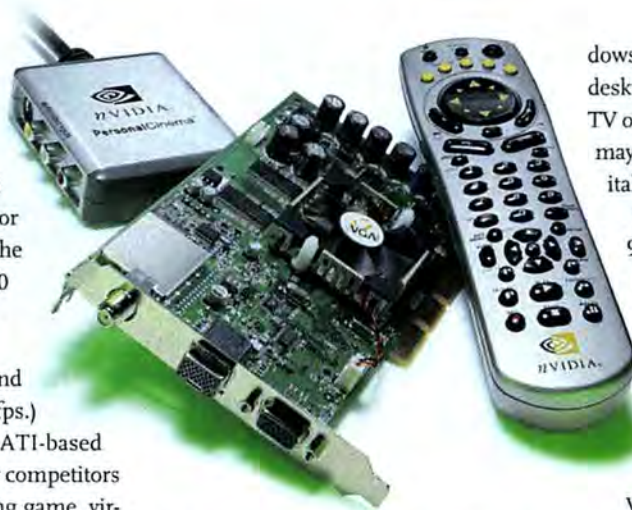
EVGA'S PERSONAL Cinema FX 5200 card comes with an RF remote and breakout box.
