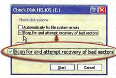
FIGURE 4: BLOCK OFF hard-disk potholes via this option in the ScanDisk utility.
