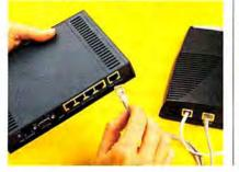
Connect the wires. If you're using a standard, wired network, plug a Category 5 network cable into the computer's network jack, and insert the other end into the hub, switch, or router. (Many wireless routers include a built-in switch that allows you to connect additional PCs using an ethernet cable.) Repeat for each connected PC.
