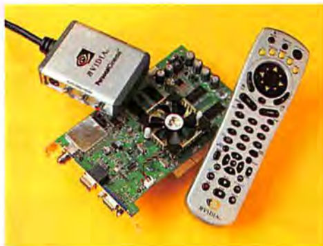
EVGA'S NVIDIA PERSONAL Cinema FX 5200 with its included remote and break-out box of connectors.
