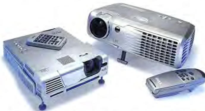
THE SUPERSLIM Plus Vision V3-131 (left) achieves its small size thanks to its pop-up lens mechanism; by contrast, Dell's 3300MP is big and boxy.
