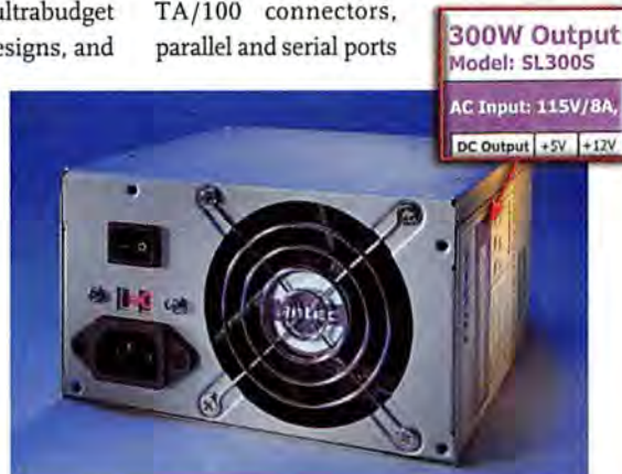
FIGURE 1: GIVE YOUR MOTHERBOARD the power it needs by upgrading to a 300-watt device such as Antec's SL300S.
