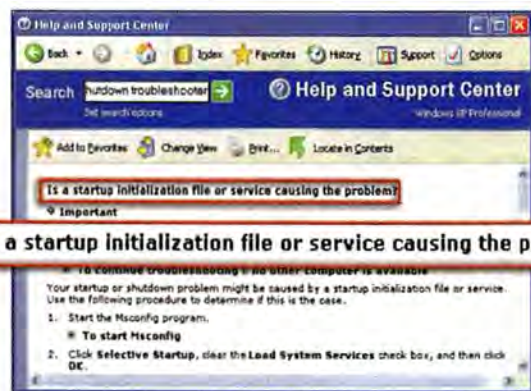
FIGURE 1: WHEN WINDOWS WON'T shut down, turn to the Startup and Shutdown Troubleshooter first.
