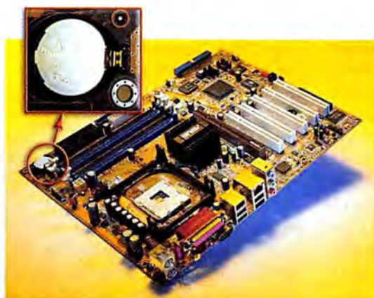
FIGURE 1: THE CMOS BATTERY on your motherboard may need to be replaced after four or five years.
