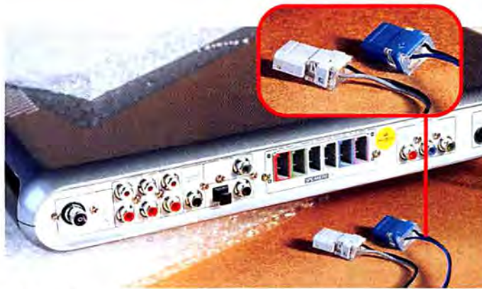
MAKING A CONNECTION: The speaker wires that come with the Philips LX3750 have large plastic terminals that are exceptionally easy to hook up.
