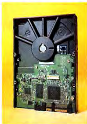
MAXTOR'S DiamondMax 10 has NCQ smarts—and a 16MB cache.
