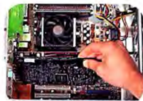
SOME PCI cards may require a bit of force to seat correctly.
