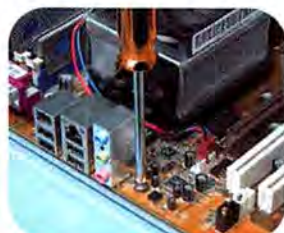
SCREWS FASTEN the motherboard onto the system case.
