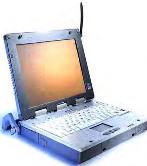
THE HP RUGGED Notebook Nr3600 has a heated screen, an illuminated keyboard, and recessed connections.
