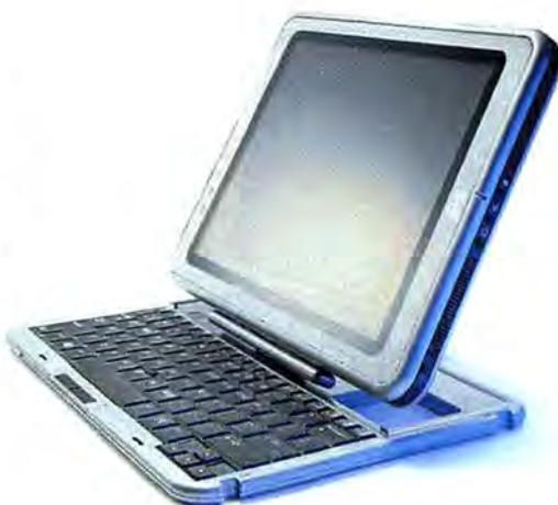
THE HP COMPAQ TABLET PC Tc1100 has a small keyboard that detaches from the touch-screen panel.
