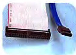
PARALLEL ATA cable (left) and Serial ATA cable.
