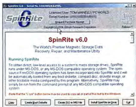
TO RUN SPINRITE version 6, you must first install it on a boot-up floppy disk, disc, or USB flash drive.
