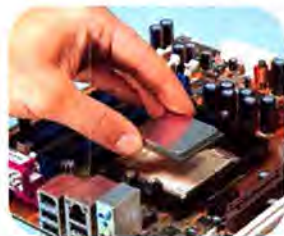
THE CPU will fit correctly into the socket in only one way.
