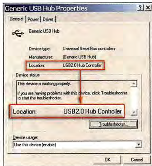
FIGURE 2: CHECK YOUR SYSTEM'S Device Manager listings for 'USB2.0' or 'Enhanced'.
