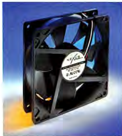
FIGURE 3: KEEP YOUR PC COOL and quiet with a slower-turning replacement fan such as the Nexus 92mm Real Silent model.
