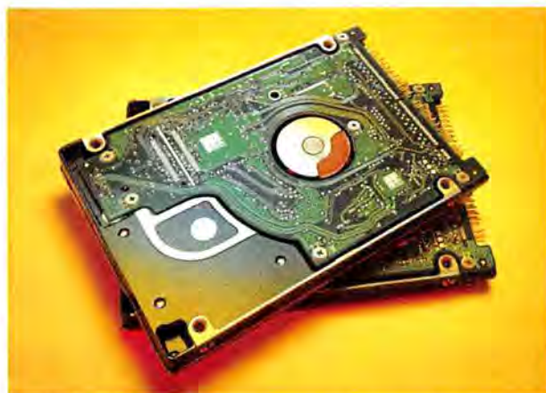
SEAGATE'S NEW 160GB Momentus 5400.3 drive with PMR technology (top) and the older 120GB Momentus 5400.2 drive.
