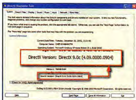
FIGURE 4: CHECK THE INSTALLED version of DirectX with the Direct X Diagnostic Tool.
