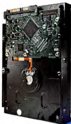
SEAGATE'S 750GB DRIVE uses perpendicular recording.
