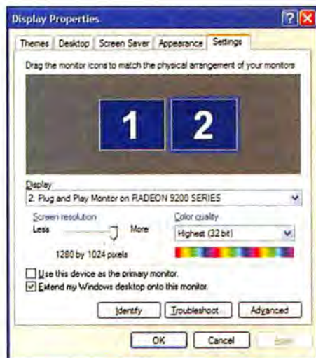
FIGURE 2: WINDOWS XP'S dual view joins your laptop's LCD with an external monitor.
