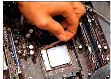
● UNLATCH and pull up the small lever to release the old CPU (step 4).
