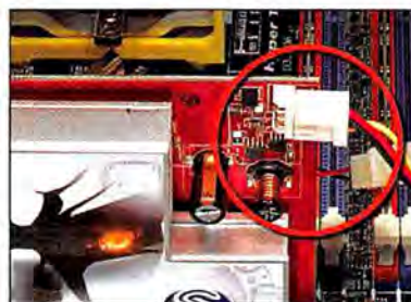
● MOST MODERN graphics cards use a dedicated power connector (step 4).
