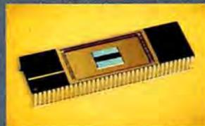
PRAM doesn't have to be erased before new data is written to it, which Samsung claims helps make it up to 30 times faster than conventional flash memory. It should also
