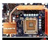
SEVERAL BOARDS FEATURE heat-pipe cooling. This is a clever way to reduce noise without using multiple fans.
