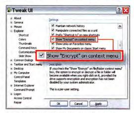
FIGURE 2: MAKE ENCRYPTION EASIER by adding a context menu command using the Tweak UI freebie.
