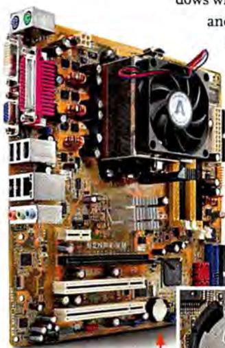
**YOUR CMOS BATTERY** may stand vertically or lie flat (as shown here) near the CMOS jumpers.
