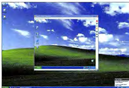
WINDOWS IN MY Windows: Parallels Workstation creates a virtual PC for trying out applications and alternative OSs.
