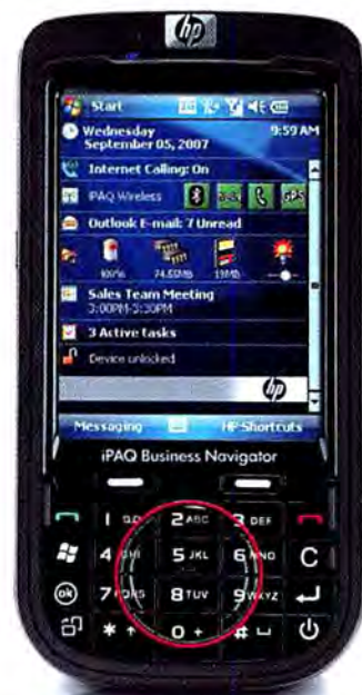
THE IPAQ 610'S on-keypad navigation wheel helps users move about the large display.
