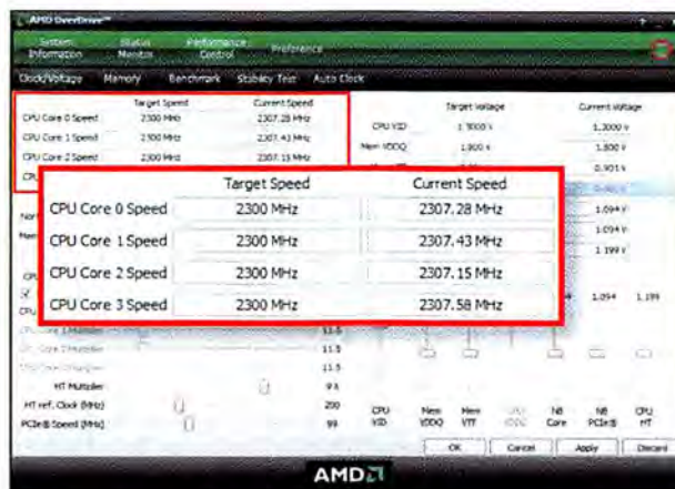
AMD'S OVERDRIVE UTILITY has an impressive array of options, letting you change multiplier and voltage settings on a per-core basis.
