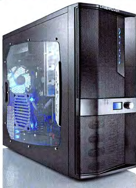
CYBERPOWER'S GAMER ULTRA CF 3870 features AMD's 2.3-GHz Phenom 9600 CPU and an ATI Radeon HD 3870 graphics board.
