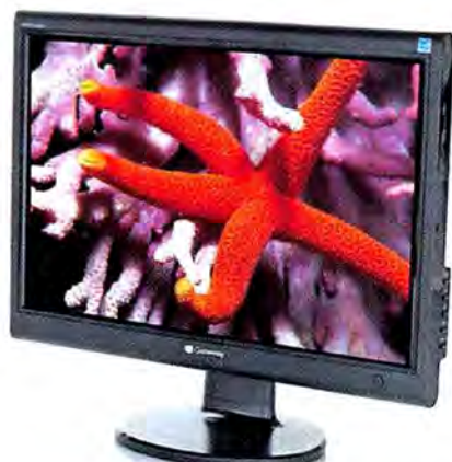
19-INCH WIDE SCREENS: Dell's $259 UltraSharp 1908WFP (left) and Gateway's $230 FPD1975W share a native resolution of 1440 by 900.
