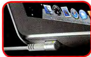
THE MAGSAFE CORD is recessed into the underside, and the adapter snugles up against the side.
