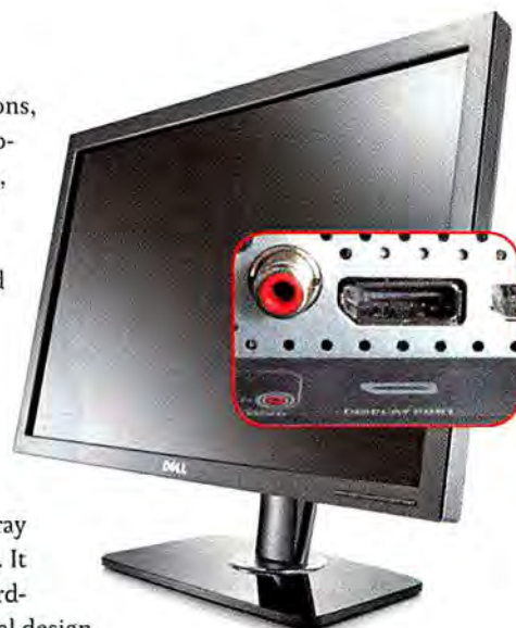
THE DIGITAL DISPLAYPORT connector is similar in size and shape to an HDMI port.
