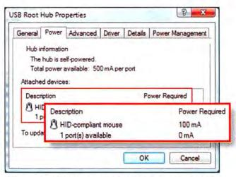
THE MOUSE ON this USB port draws 100 milliamps of power. Add the totals for all devices to confirm that you have enough power.
