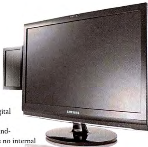
THE SECONDARY LCD connects to the main display via USB.
