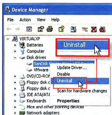
IF WINDOWS CAN'T see a USB drive, uninstall it via Device Manager, unplug, and replug.
