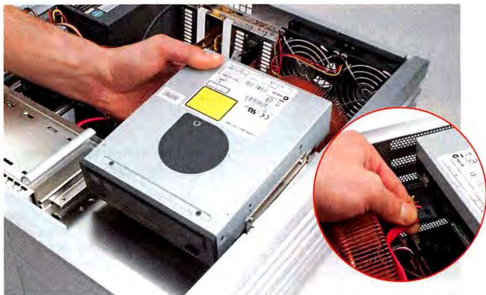
WHAT WOULD a high-definition computer system be without a Blu-ray Disc drive installed? The Pioneer BDC-2202 comes equipped with a SATA interface (see inset), just as your internal hard drive does.
