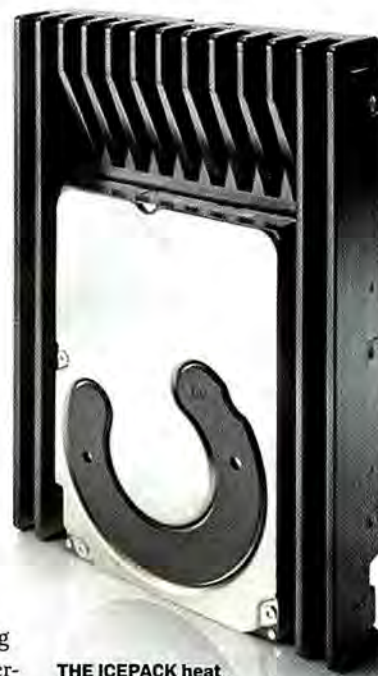
THE ICEPACK heat sink on the VelociRaptor keeps the drive cool—and makes it easy to mount in a PC.
