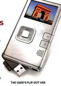
THE VADO'S FLIP-OUT USB connector can make attaching the camera to a PC difficult.
