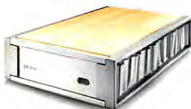
THE REDRIVE HAS a bamboo top, and heat sinks on its sides.
