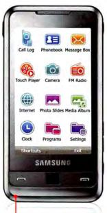
SAMSUNG'S OMNIA HAS a 3.2-inch WQVGA screen (which is slightly smaller than the iPhone's) and an optical mouse for navigation. It sports a 5-megapixel camera, too.
