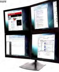
nector. Link the upper-left monitor to the primary connector on the second graphics board, and the upperright screen to the remaining connector. This arrangement will make it easier to configure the screens in Windows.
