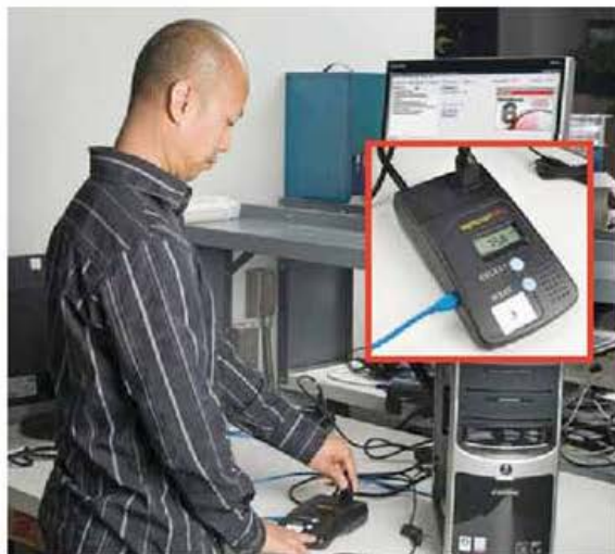
PC WORLD DEVELOPMENT Analyst Thomas Luong uses a Watts Up meter to measure a system's power draw at various states.
