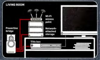
for devices that are stationary and need a consistent network connection. Plug another powerline bridge into a wall socket, and you can run an ethernet connection to a set-top box (such as a TiVo) or to a network-attached storage device. You can even connect to a Wi-Fi access point if you have trouble getting a signal from your main router.
