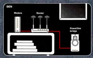
THE EXTRA PIECES of a powerline network are two powerline bridges and cabling. The network starts in whatever room houses your router. You connect the powerline bridge to a wall socket (not to a power strip), and then you run an ethernet cord from the bridge to one of the ports of your router. Powerline networks are most useful
