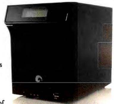
**SEAGATE'S BLACK ARMOR NAS 440 provides data-redundancy options over a network.**
