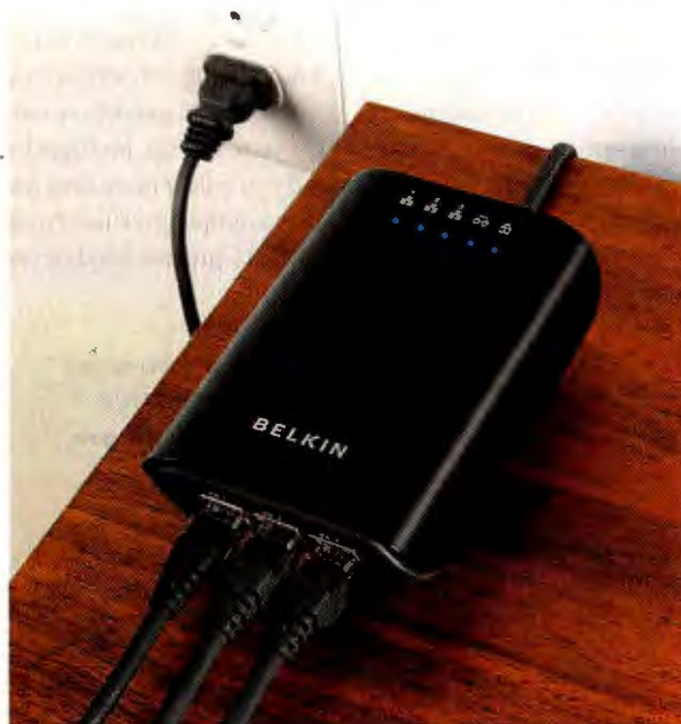
THE BELKIN POWERLINE AV+ Starter Kit has the basic hardware you need to transmit TV signals through your home's electrical wiring.
