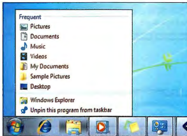
WINDOWS 7'S NEW TASKBAR sports better thumbnail previews, context-sensitive Jump Lists, and other features that help speed up the navigation and management of applications and windows.
