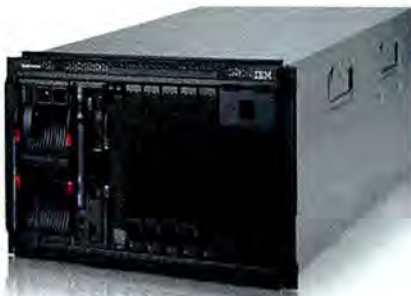
A SINGLE IBM Blade Center S chassis with six blades replaced a system of 12 servers.
