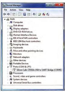
MAKE SURE THE ports are correctly assigned in Device Manager—this controller is on COM4.
