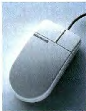
At 400 ppi, Microsoft's new mouse has twice the resolution and faster on-screen movement than previous versions.
