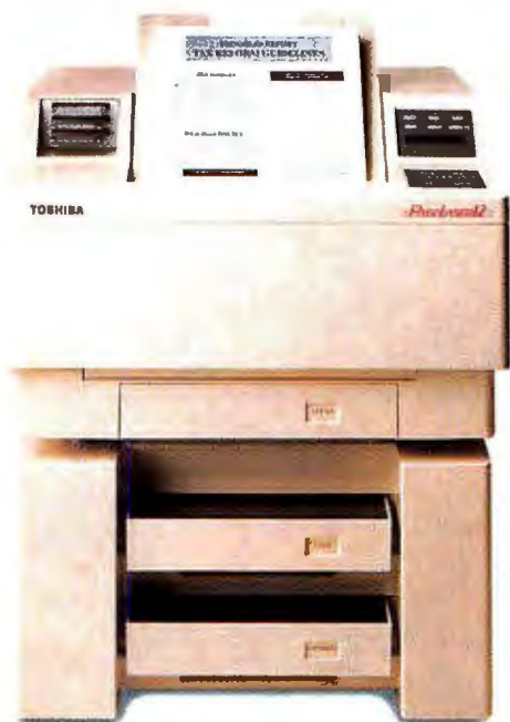
Page Laser12: 12 ppm, up to 3 paper bins, 750 sheet capacity, Toshiba/Qume, Diablo, IBM & HP emulations.
