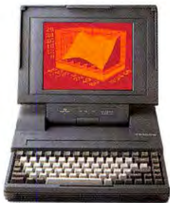
T3100e: 12MHz 80286, internal IBM slot, 20MB hard disk, gas plasma display, 1MB RAM expands to 5MB, 1.44MB 3½" diskette drive.
