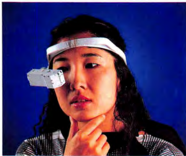
The Private Eye provides computer users on the go with the equivalent of a 12-inch screen that fits in a pocket.
