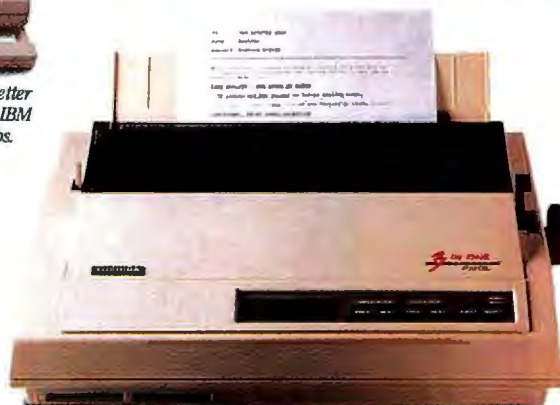
P321SL/SCL (color): 216/72 cps, 24-pin letter quality, up to 360x360 DPI graphics, Toshiba/Qume and IBM emulations standard, Epson and Diablo emulations optional, 32KB print buffer, front panel controls, advanced paper handling.
