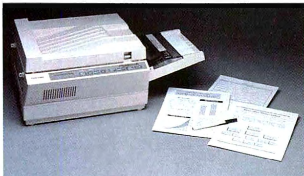
The PageLaser6, a work-group printer that uses HP LaserJet Series II fonts, is 35 percent smaller and, at 6 ppm, only a little slower than the LaserJet.
