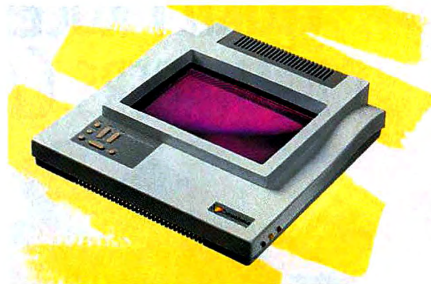
No more dim purple images—the 480C PC Viewer is the first true-color LCD overhead projection panel, fitting atop any standard overhead projector so that you can demonstrate graphics in eight vivid colors.
